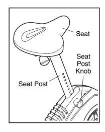
in one of the adjustment holes in the seat post. Then, turn the knob clockwise to tighten it.
