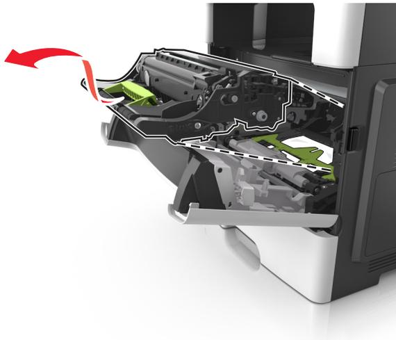
**Warning—Potential Damage:** Do not touch the shiny blue photoconductor drum under the imaging unit. Doing so may affect the quality of future print jobs.
