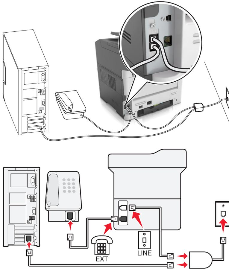
A Digital Subscriber Line splits your regular telephone line into two channels: voice and Internet. Telephone and fax signals travel through the voice channel, and Internet signals pass through the other channel. This way, you can use the same line for analog voice calls (including faxes) and digital Internet access.
