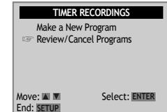
**2** Confirm reservation-recording details in turn with [V] button and then, press [CLEAR] button on the position of the details to delete.
