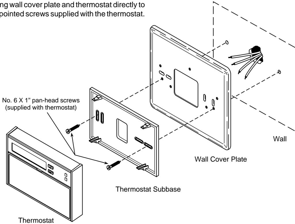
Figure 3. Mounting 1F9X digital thermostat to wall
