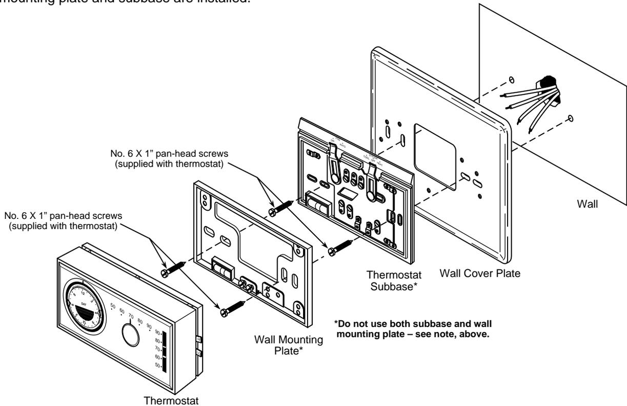
**Figure 6. Mounting 1F7X quartz clock thermostat to wall**
