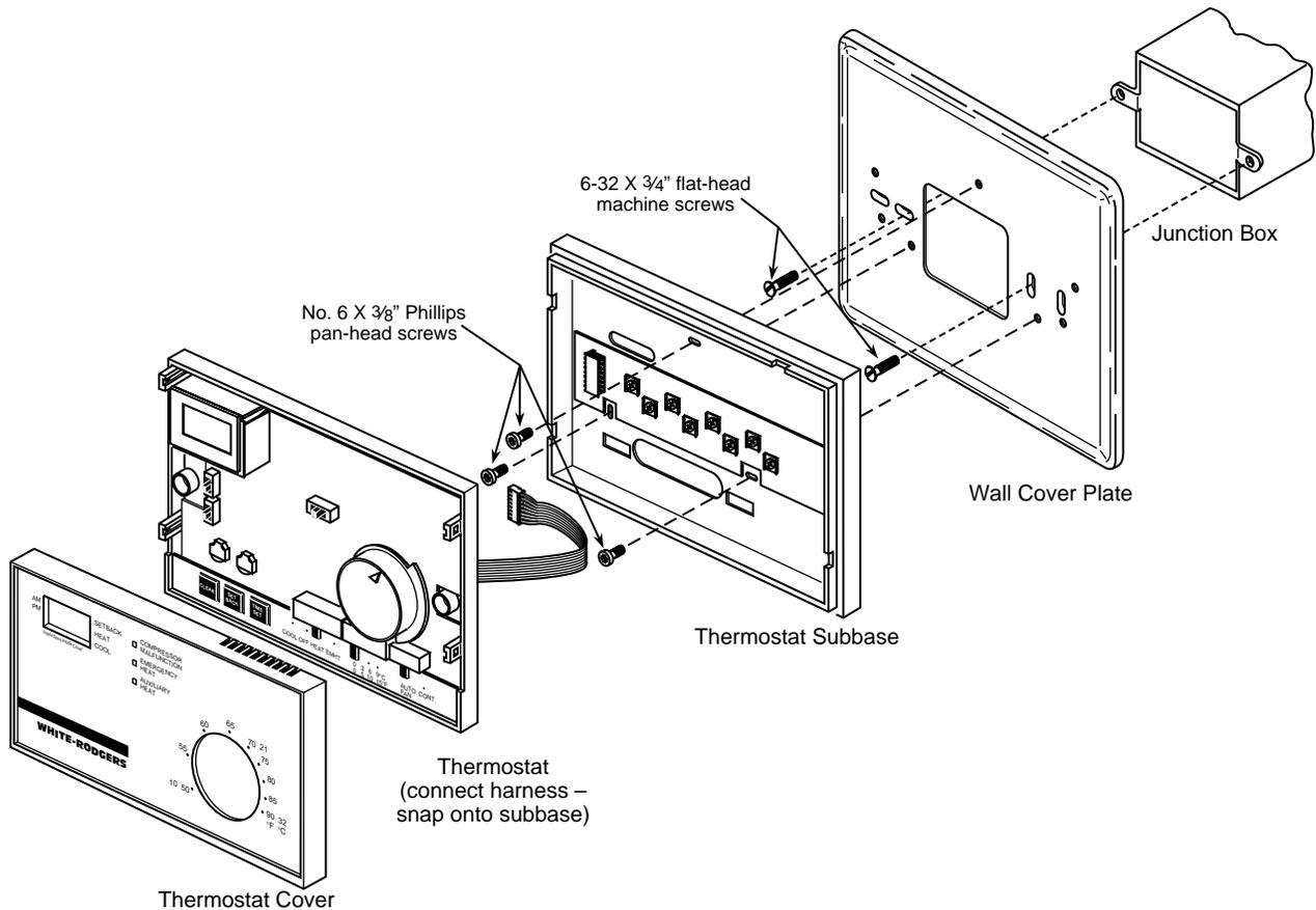
**Figure 10. Mounting 1F62 thermostat to horizontal junction box**
