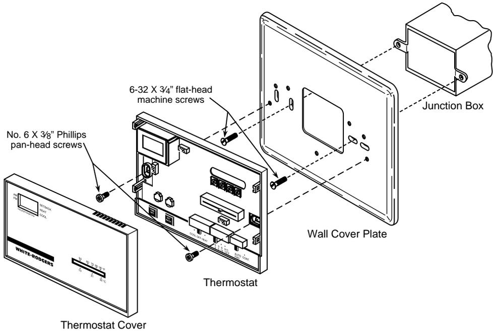
**Figure 7. Mounting 1F60 thermostat to horizontal junction box**
