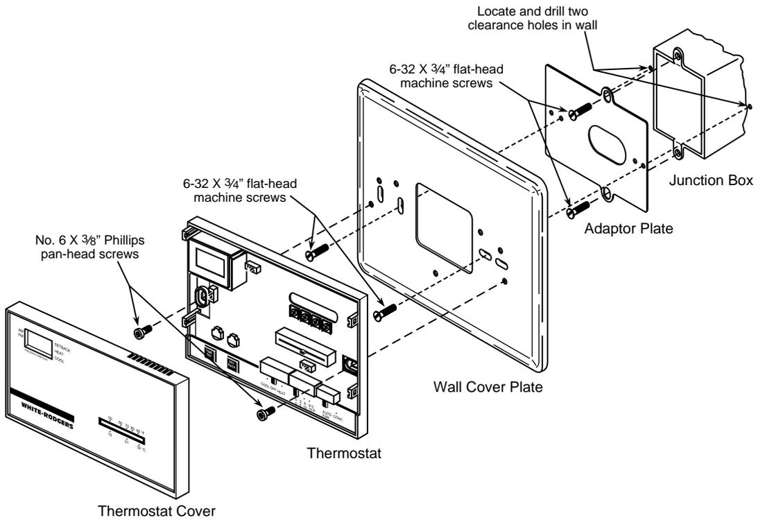
**Figure 8. Mounting 1F60 thermostat to vertical junction box**
