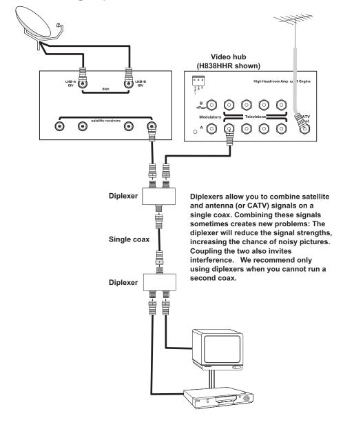
Typical room - phone, TV, ethernet, satellite receiver, AV modulators, hi-speed data Media center - phone, TV, ethernet, satellite receiver, cable modem, hi-speed data Home office -
