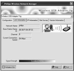
The **Link information tab** displays information on the wireless network name (Network Name) to which there is a wireless connection, the signal strength and link quality, the connection speed, the channel and the number of transmitted/received (Tx/Rx) fragments.
