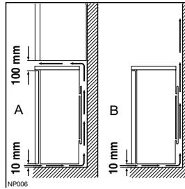
There should also be a gap of 25 mm either side of the appliance. Do not obstruct the space underneath. The back of the cabinet may be placed close to the wall but must not touch it. **DO NOT** install in places with restricted ventilation.
