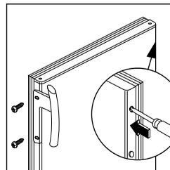
Fix the handle on the opposite side, insert the plastic plugs into the holes left open that can be found in the instruction for use bag.
