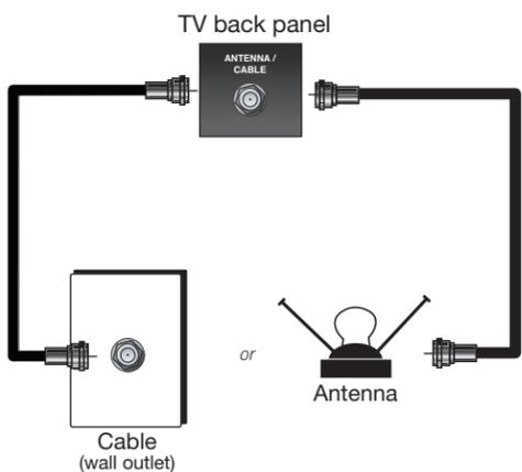
Connect your regular cable to the TV's ANTENNA/CABLE INPUT to receive analog channels or connect an antenna to the TV's ANTENNA/CABLE INPUT to receive off-air local digital and analog channels.
