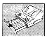
Then: Slide the cassette into the slot until you hear it lock into place.
