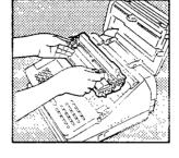
...Insert the process unit First slide the green lock lever on the inside left of the machine to the back. The process unit is then inserted with its pins into the lateral guides and placed exactly in position by applying slight pressure downwards. Now pull the lock lever forward
