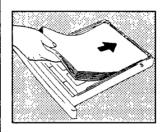
Insert a stack of A4 paper Prepare the recording paper by flexing and fanning out the stack to separate the sheets. Place the paper so that it lies straight in the cassette with the side to be printed facedown and don't forget:
