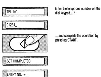
\* If you wish to programme pauses (e.g. for overseas numbers) between the STD code and the subscriber number, press PAUSE. Pauses are shown on the LCD display as hyphens. You may also enter a space between digits in telephone numbers with the # key.
