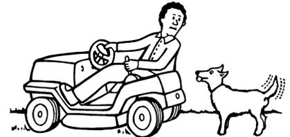
Before you leave the mower, stop the engine. Remove the key. Disengage and lower any attachment. Set the parking brake. Never mount or dismount from the seat while the engine is running. An accident can occur if you touch the brake, shift lever, throttle, clutch or blade control while the engine is running. Mount and dismount from the seat on the side of the unit that is marked ENTER-EXIT.
