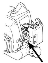
**Start throttle:** Set the throttle to the start position by first pressing the throttle lockout and the throttle trigger, then pressing the start throttle button (A). Then release the throttle lockout and the throttle trigger, followed by the start throttle button. The throttle function is now activated. To return the engine to idle, press the throttle lockout and throttle trigger again.
