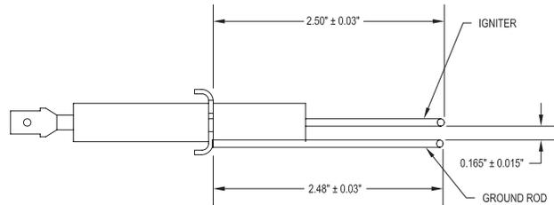
Figure 30. Direct Spark Igniter.
