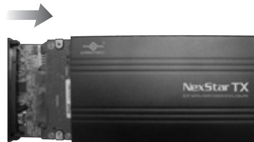
5-3 Secure the caddy to the housing using the screws provided.
