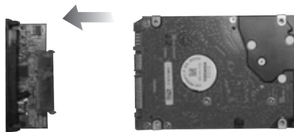
5-2 Insert the hard drive caddy back into the NexStar TX housing as the picture below. Be sure to align the caddy with the guides within the housing.
