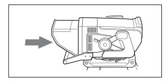
**3** Turn the viewfinder counterclockwise. Then turn the panning lock lever counterclockwise to lock the viewfinder in place.
