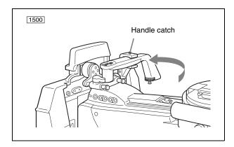
While pulling the release knob ① on the left side to release the viewfinder table, slide the table as 2 to an appropriate position. Then push the lock lever ③ toward the front to lock the viewfinder table in place.
