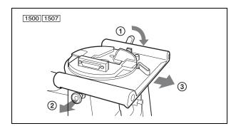
**3** Push the rear panel lock release lever on the left panel down to open the rear panel.
