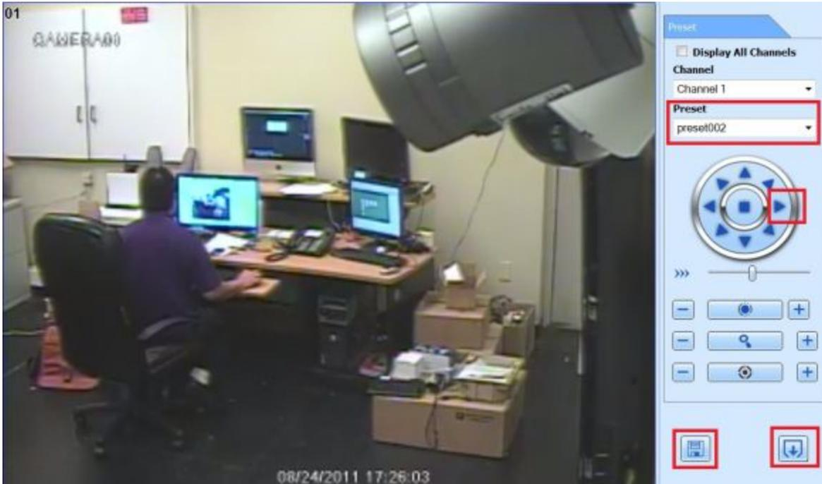
6. Go back to the main camera live screen and select Preset 101 and click on Enter button to start moving the camera from left to right and back and forth.
