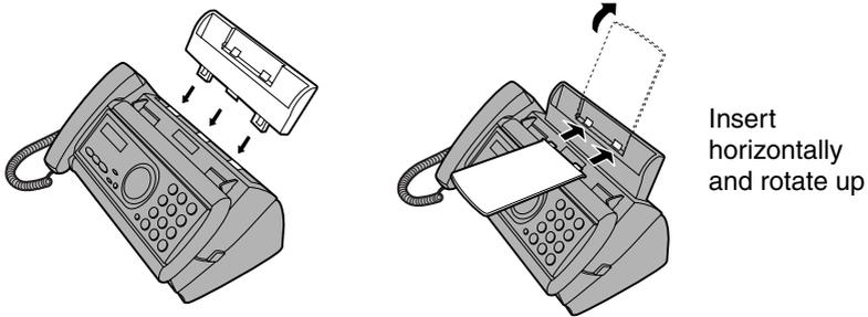
**Note:** The paper tray extension has a top side and a bottom side. If you cannot insert the tabs into the holes, turn the support over.
