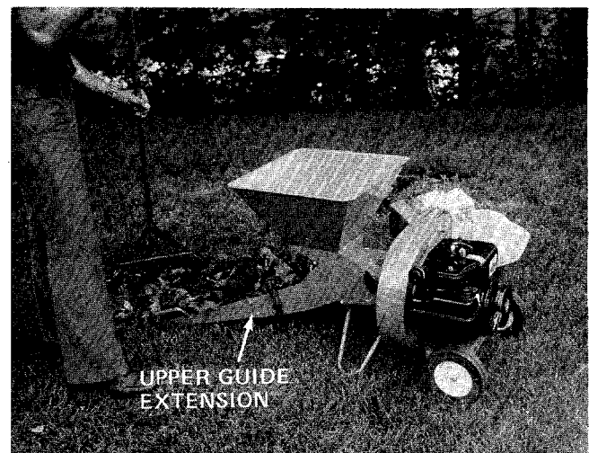
FIGURE 11. RAKING LEAVES AND TWIGS INTO UPPER GUIDE EXTENSION
