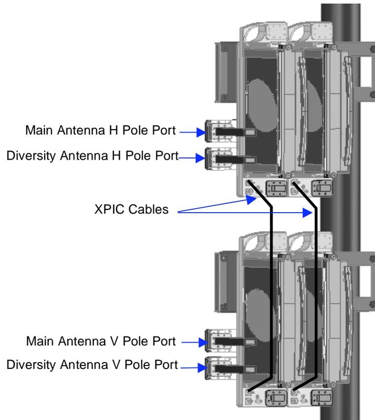
8. Connect the flexible waveguides to the antennas, as shown in the illustration above (V and H poles are selected as required - in the illustration above they are selected arbitrarily).
