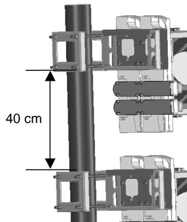
**Important:** The diameter of the pole upon which the kit is mounted must be between 50 mm (2") and 125 mm (5").
