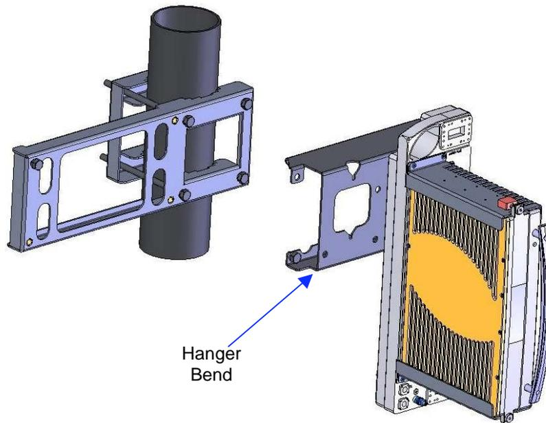
Side view showing how the Hanger Kit is hung on the Pole Mount Kit.
