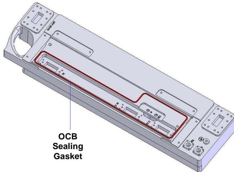
3. Gently slide the RFU in the OCB, making sure that the two empty spaces in the RFU correspond to the filter positions on the OCB.
