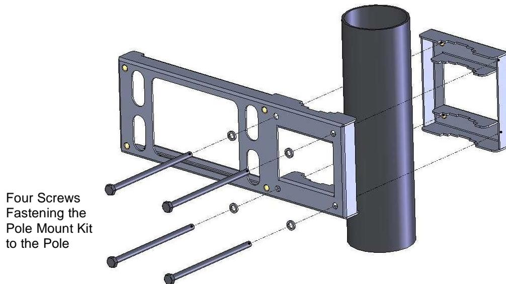
2. Fasten the kit to the pole using the 4 screws, as shown in the photo above.
