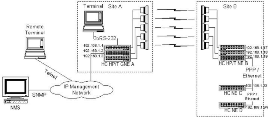
Each IDC calculates its own IP address, considering cascade shelf# and floor#:  $IP = IPbase + 3 * shelf\# + floor\#$
