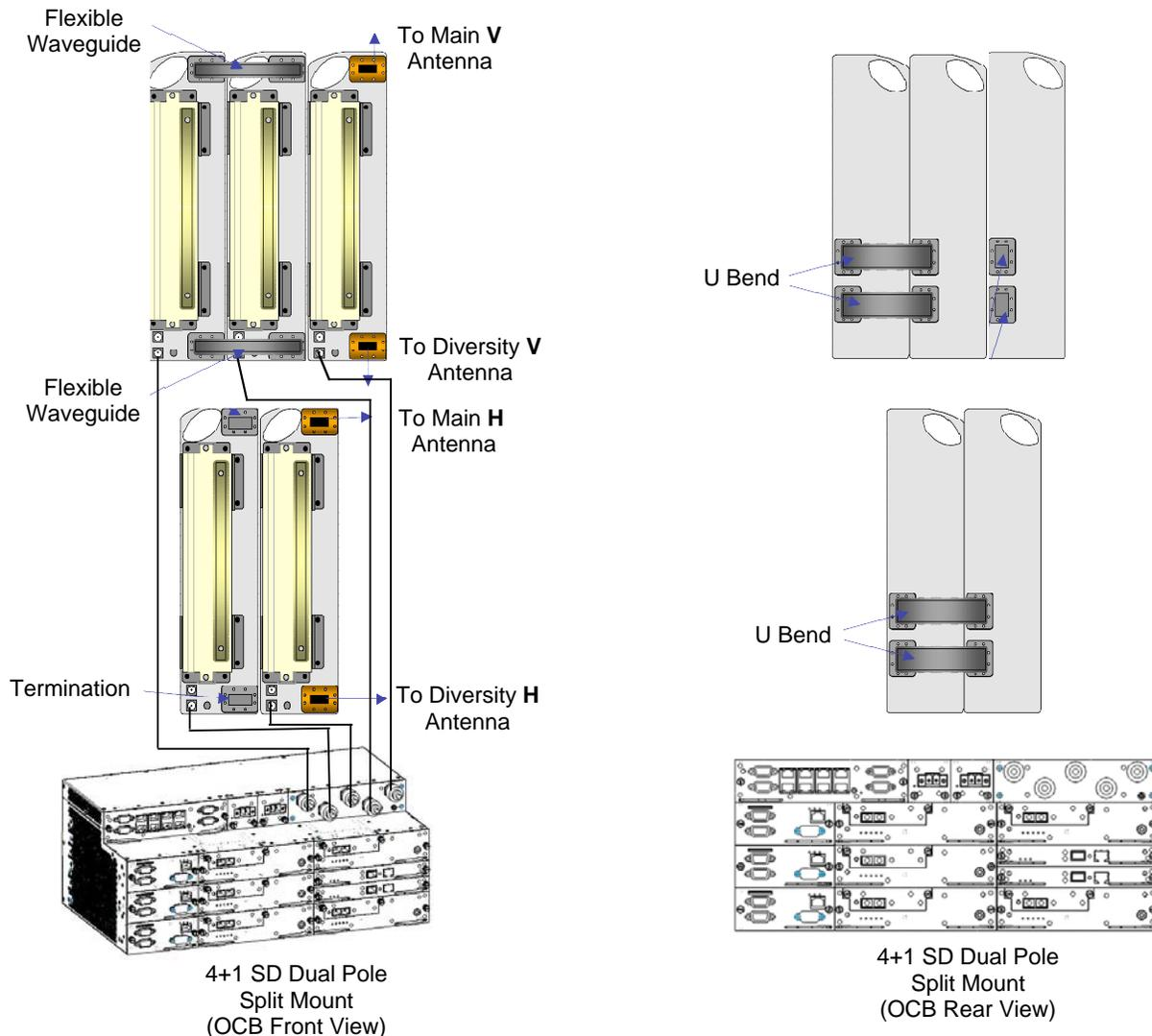
**Note:** When installing an N+1 configuration, assemble the OCBs in an inverted order, to maintain the same branching loss between the carriers, as shown in the following illustration.
