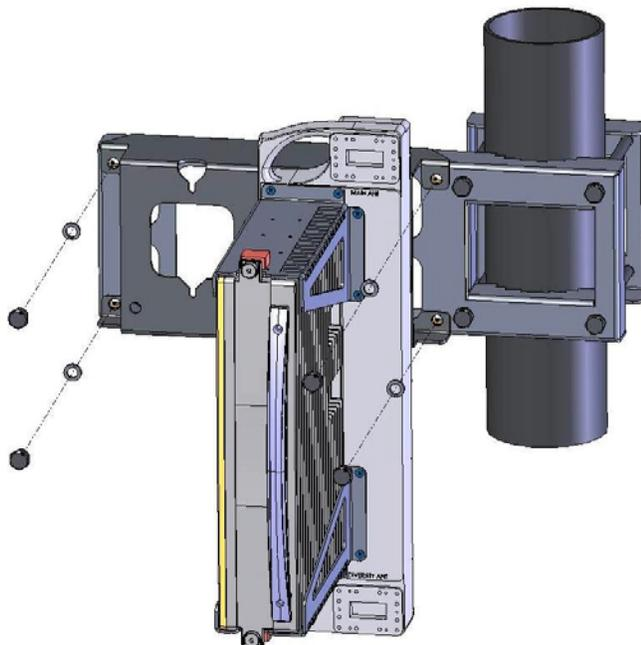
Each Pole Mount Kit can accommodate two RFUs and OCB units, as shown in the following illustration.
