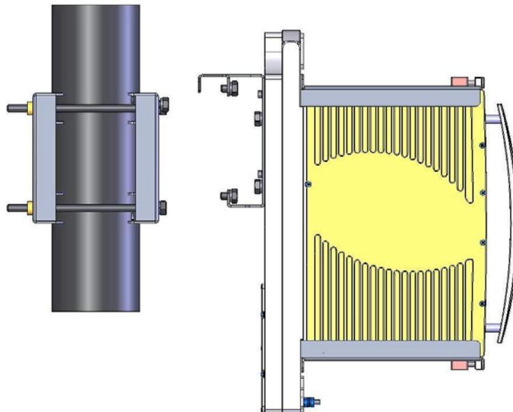
Side view of the Hanger Kit assembled on the Pole Mount Kit.
