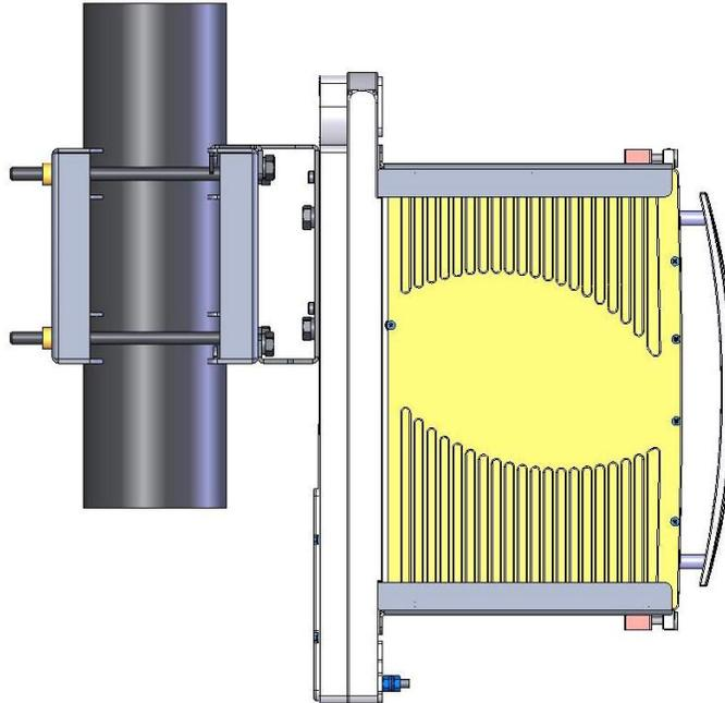
2. Fasten the Hanger Kit to the Pole Mount Kit using 4 large (M-10 type) screws, as shown in the following illustration.
