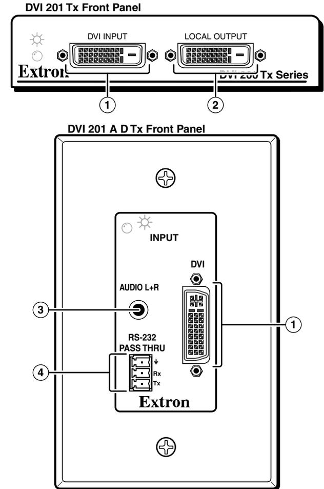
**Figure 2-12 — DVI 201 Tx front panel connectors**
