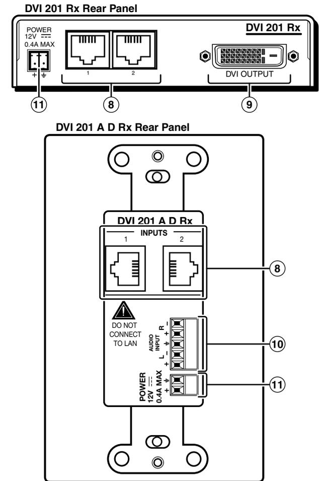
**Figure 2-16 — DVI 201 Rx rear panel connectors**
