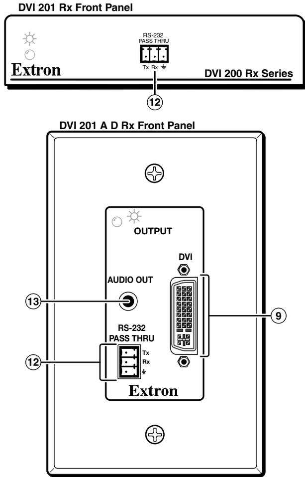
**Figure 2-17 — DVI 201 Rx front panel connectors**
