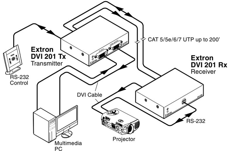
**Figure 1-1 — Typical transmitter and receiver application**
