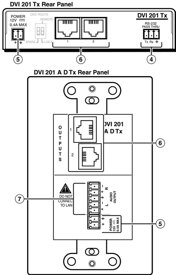
**Figure 2-13 — DVI 201 Tx rear panel connectors**
