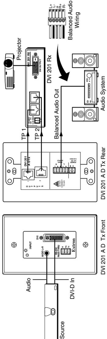
**Figure 2-28 — Typical installation**
