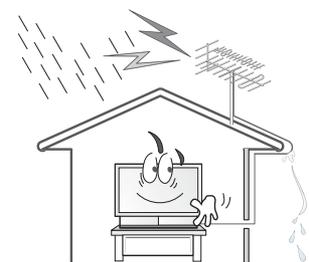
**Any necessary action such as making the antenna cable loop at the entrance of the building should be taken to prevent rainwater on the outdoor antenna cable from possibly running into the indoor.**
