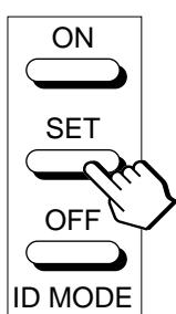
You can operate only a specified monitor. (All operations are available in ID mode except POWER ON/OFF.)
