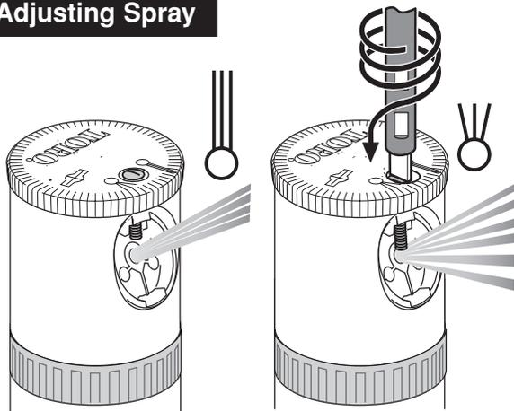
Turn the nozzle screw in to diffuse and shorten the spray radius.
