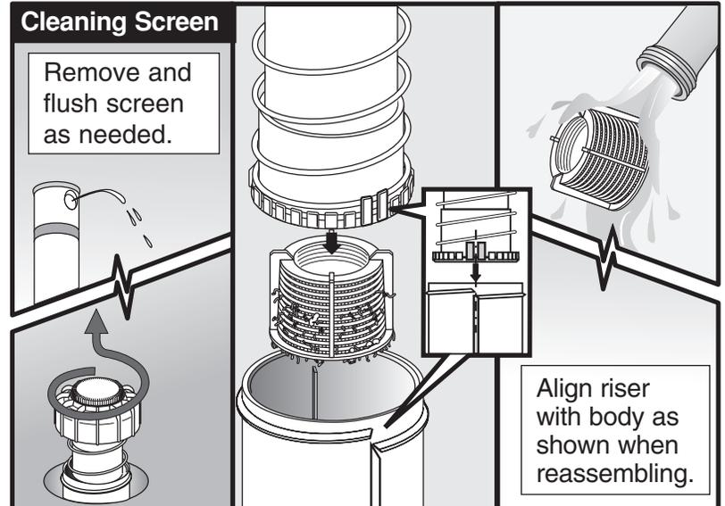
Align riser with body as shown when reassembling.
