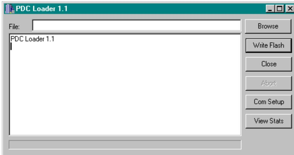
Ensure your PC and DL are properly connected, see *Setting Up At The Office, Page 15*. The serial data cable should go from any COM port on the PC to COM2 on the DL. Have all power cables in place but do not turn on the DL just yet. Power the DL using the AC adapter. Do not use batteries, as power interruptions during the process may damage the DL, see the warning below.
