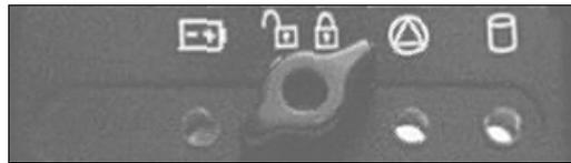
*Table 4* shows what the colors of each indicator signify. When the DL is connected to two batteries, the Power indicator is pulsed (in the appropriate color) to distinguish between battery A and battery B. One long “blink” corresponds to battery A, and two short blinks in rapid succession correspond to battery B. Only the status of the active battery is indicated.
