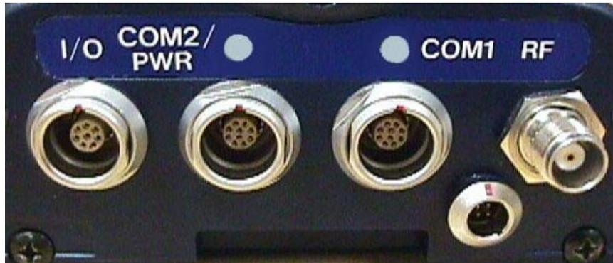
Each connector is keyed to ensure that the cable can be inserted in only one way, to prevent damage to both the DL and the cables. Furthermore, the connectors that are used to mate the cables to the DL have a locking mechanism that requires careful insertion and removal. Observe the following when handling the cables.
