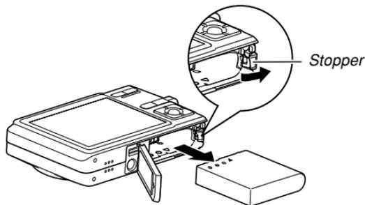
3. Release the stopper and pull the battery from the camera.
