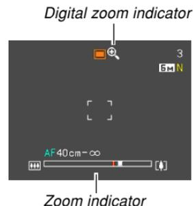
2. When the zoom pointer reaches the optical/digital zoom switch over point, it will stop.
