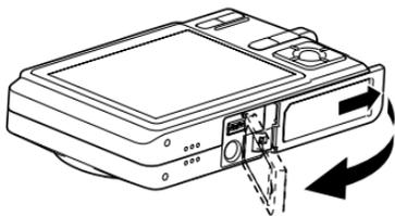
2. While pulling the stopper in the direction indicated by the arrow in the illustration, align the arrow mark on the battery with the arrow mark on the camera and slide the battery into the camera.
