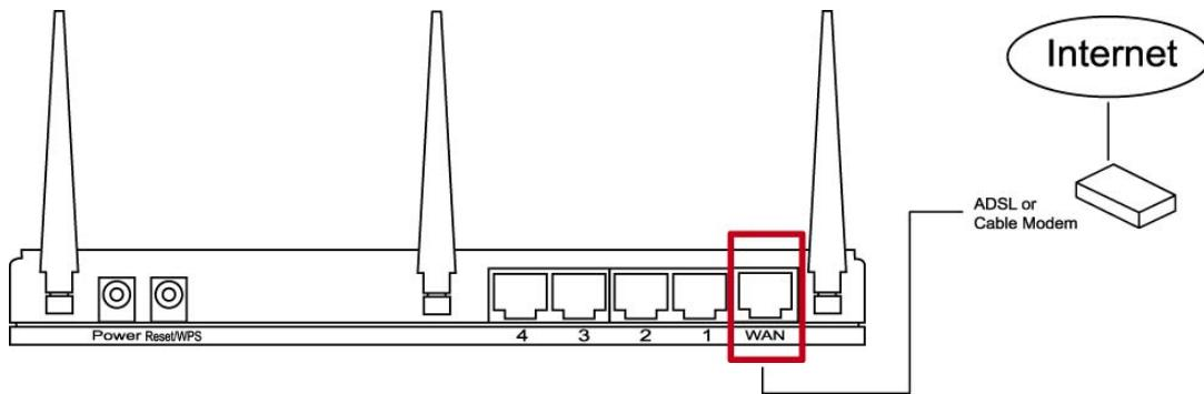
2. Connect all your computers, network devices (network-enabled consumer devices other than computers, like game console, or switch / hub) to the LAN port of the router.
