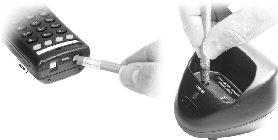
Figure 9: Cleaning the Battery Charger Contacts
