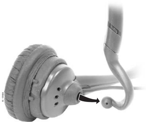
Figure 17: Installing the Optional Earloop
