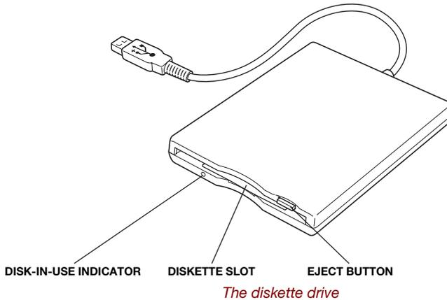
An externally connected 3 1/2" diskette drive lets you use either double density (720 KB) or high density (1.44 MB) 3 1/2" diskettes for data transfer and storage.
