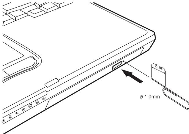
*Manual release with the eject hole*
