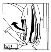
Removal of fluff will be made easier if you moisten your hand or use a damp cloth. After cleaning, fold down the coarse filter and reengage it securely.
