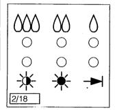
I am provided with an electronic degree of dryness indicator on programmes 1 − 8. The symbol lighting up in each case shows you the degree of dryness attained by your laundry. Symbol → additionally lights up at the programme end.
