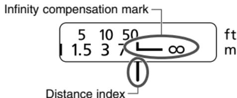
To compensate for shifting of the infinity focus point that results from changes in temperature. The infinity position at normal temperature is the point at which the vertical line of the L mark is aligned with the distance indicator on the distance scale.
