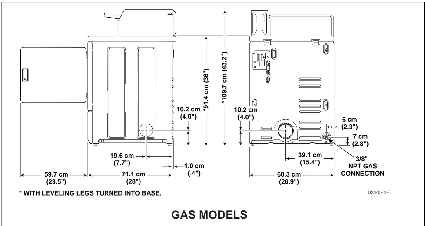
**NOTE:** Side, rear and bottom exhaust openings are 10.2 cm (four inch) ducting. Gas models cannot be vented out left side of cabinet because of burner housing.
