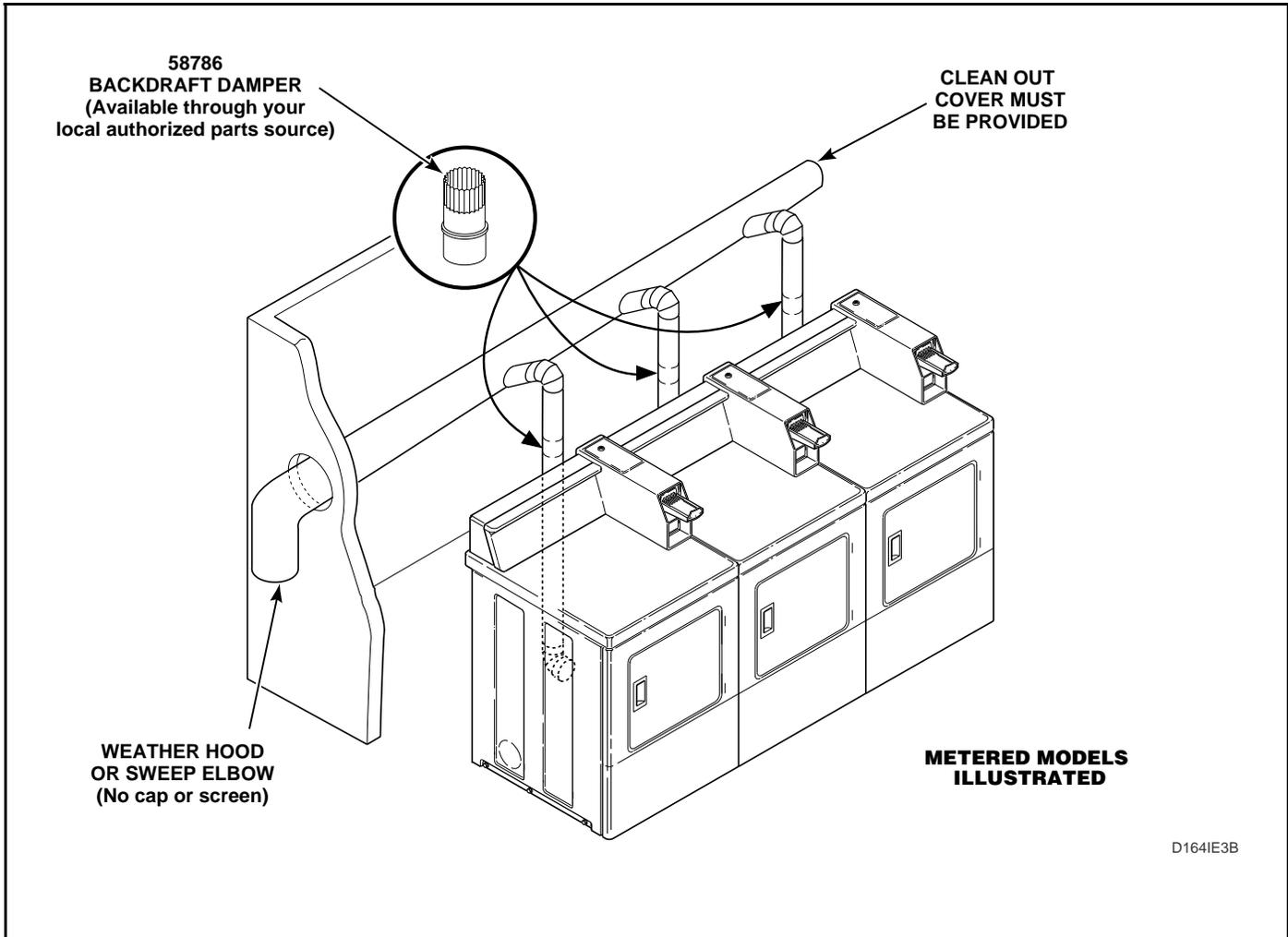
**IMPORTANT:** Static pressure in the dryer's exhaust duct should be no greater than that shown in the chart on Page 23. This can be measured with a manometer placed on the exhaust duct approximately 60.96 cm (two feet) from the dryer. See Page 23. All dryers connected to the main collector duct should be in operation when pressure is checked.
