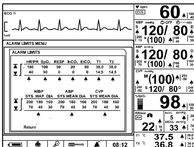
Figure 17. Alarm Limits Setting
