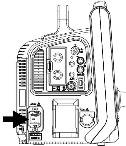
**Figure 6. AC Power connection**
