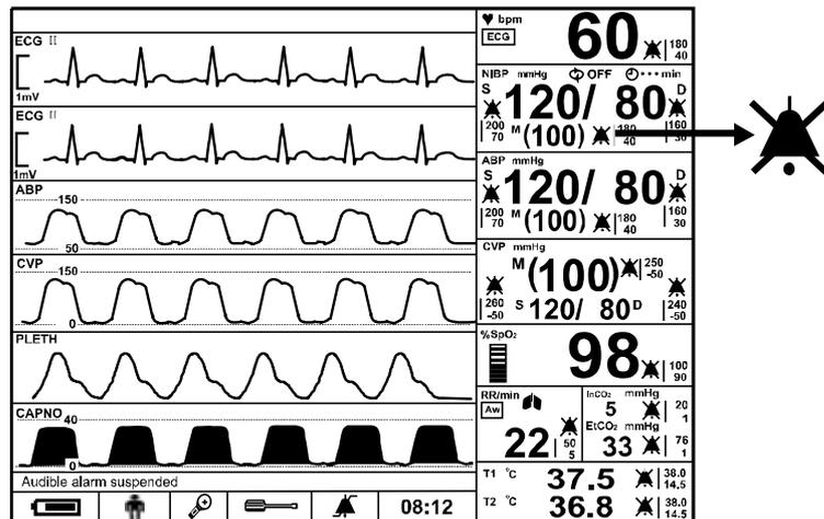
Figure 20. Audible Alarm Suspend Display
