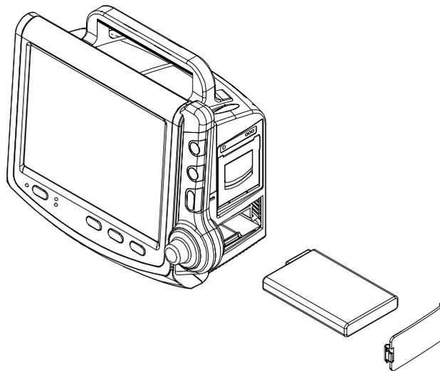
**Figure 7. Battery Placement**
