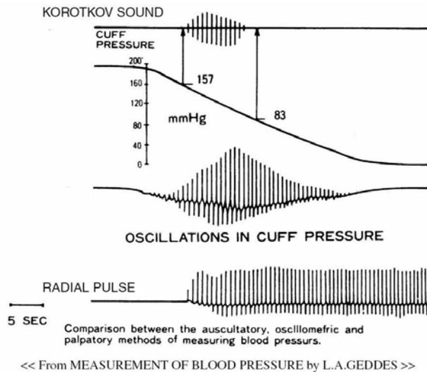
The oscillometric method does not determine an instantaneous blood pressure reading like the auscultatory method employing a microphone-type auto blood pressure monitor but, as described above, determines blood pressure from an uninterrupted changing curve, which means that the oscillometric method is not easily effected by external noise and electrosurgical instruments.
