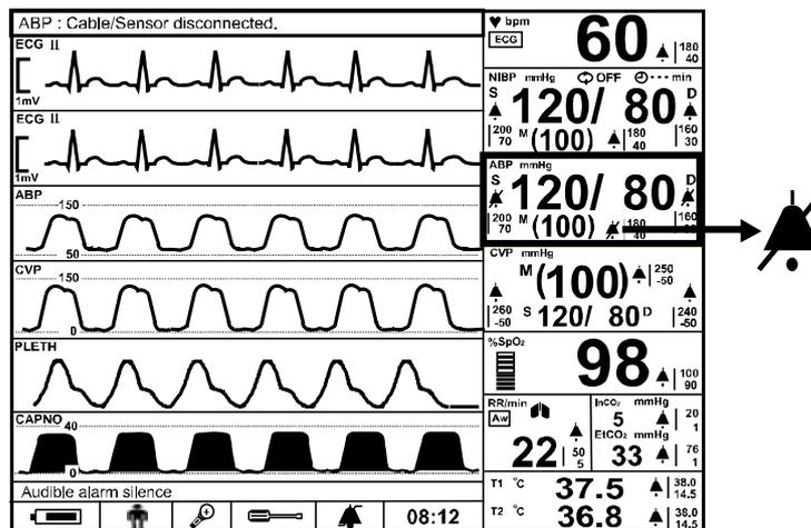
Figure 19. Audible Alarm Silence Display
