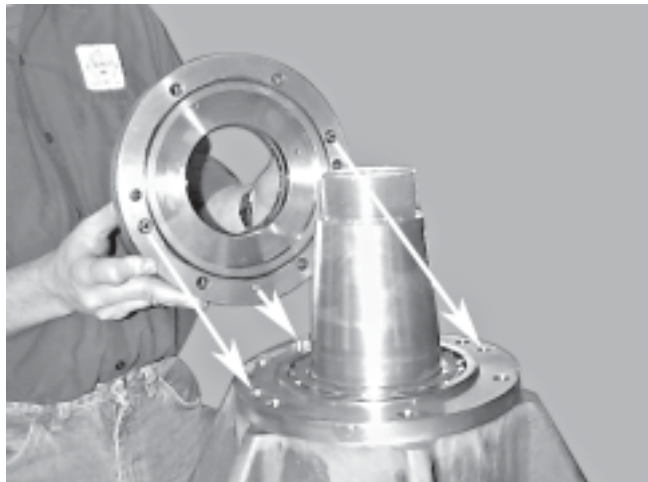
Aligned oil and grease openings and alignment dowel in the upper seal plate
