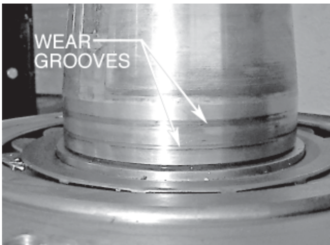
Grooves in shaft caused by seals
