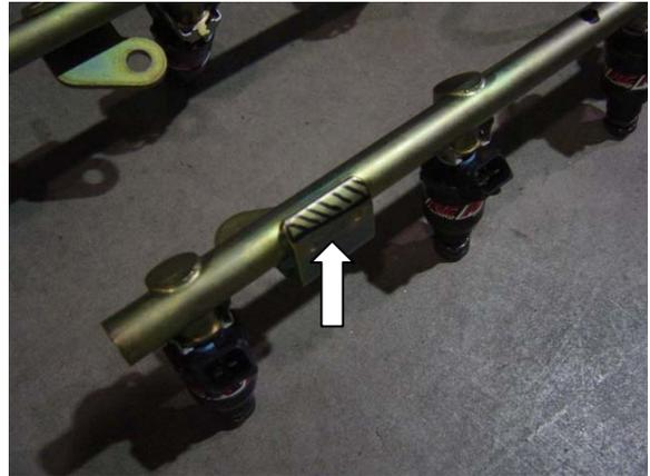
3. Install the 440cc injectors and reinstall the fuel rail using the provided spacer. (Part Used #65)
