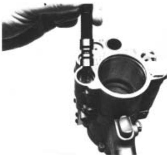
2. Remove feed control valve assembly with threaded rod (7/16-20).
