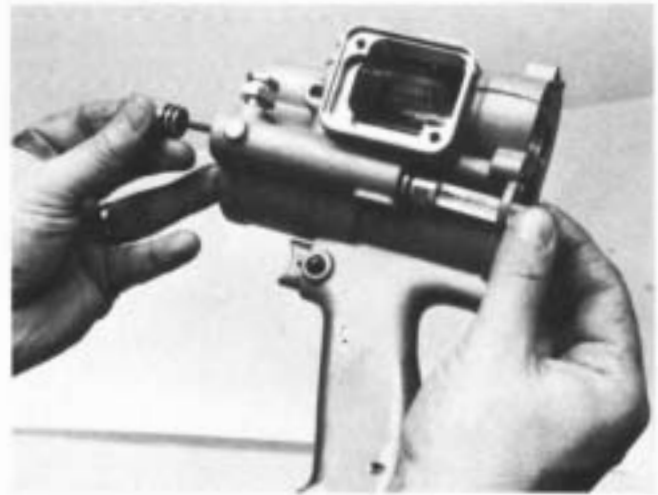
4. When reassembling, the oil indicator guide must be inserted from the rear of the tool, and the indicator piston and rod assembly must be inserted from the front of the tool as shown. Failure to follow reassembly instructions will result in damaged O-rings.
