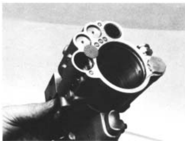
3. Remove pipe plug from rear of feed adjust boss and push forward to remove filter and O-ring.
