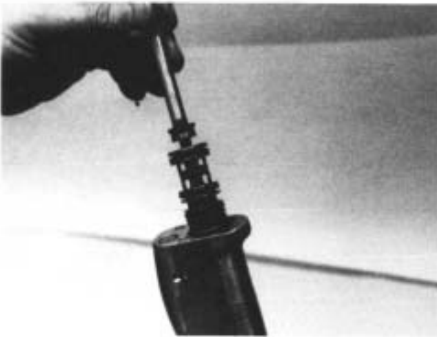
3 Insert long 8-32 screw into tapped hole provided in base of pilot spool and lift out. NOTE: Be careful not to bend pilot spool when removing or inserting. A bent spool will cause the tool to malfunction and will require spool replacement.
