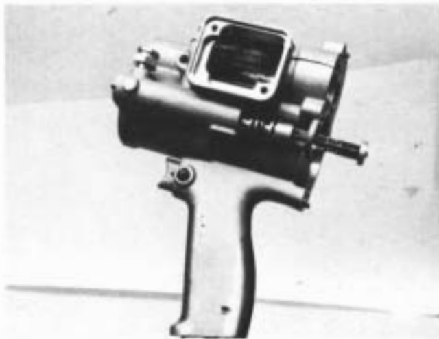
3. With suitable driver, drive out oil indicator guide, piston and rod assembly through the rear of the housing. Caution: Do not score or scratch inside of bore with driver.
