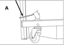
Press Brake Lever DOWN to engage braking mechanism for front castor located directly below the Brake Lever.
