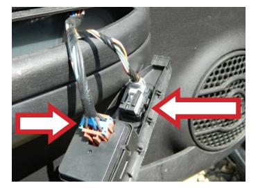
**STEP 15:** Install the master power switch assembly into the interior door trim panel.
