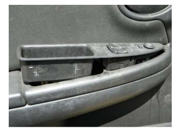
**STEP 5:** Disconnect the master power switch assembly from the door harness.
