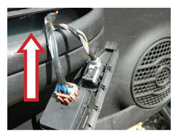
**STEP 13:** Install the interior door trim panel, be sure to align all of the interior door trim panel retainers before pressing the panel into place.
