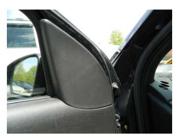
**STEP 3:** Remove the master power switch/ interior door trim panel attaching screws.
