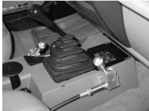
Mount the shifter(s) in an easy to reach and easy to maintain place and in a straight as possible path with the cable (do not kink the cable).
