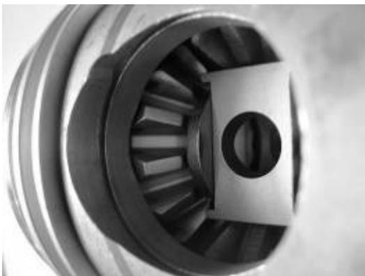
Push axles in and install the c-clips, once this is done pull axles out some until they are properly in place
