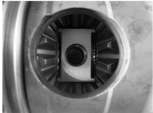
Rotate the carrier with opened end facing out so that you can install the c-clips.
