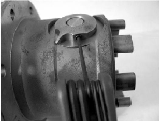
Install the dowel pin and then the set screw. Add High Strength Lock-tite to the set screw prior to installation.
