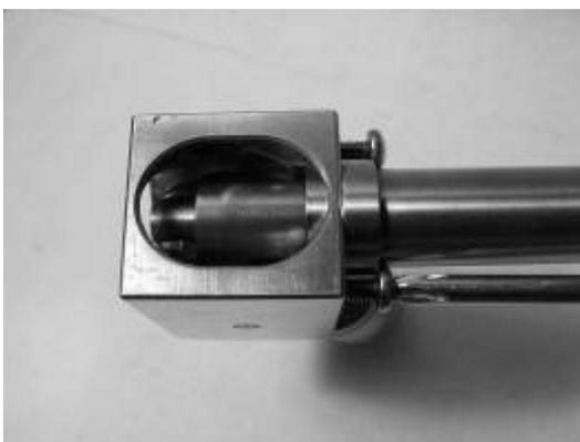
Shift several times into lock and unlock. Check the shift on the unlock position (make sure it is still touching, if not adjust appropriately, then tighten the two screws on the swivel fitting, tighten the lock nut, and install your shifter.
