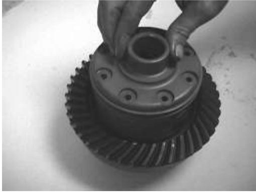
Install small carrier cap – align holes, make sure it slides into locking side gear smoothly. **NOTE: Make sure this cap sits flush with all 8 cams – if cap is not flush, it could cause severe damage to the carrier**
