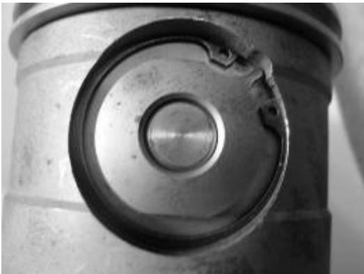
Install the snap ring into the groove. Make sure snap ring is fully seated into groove.
