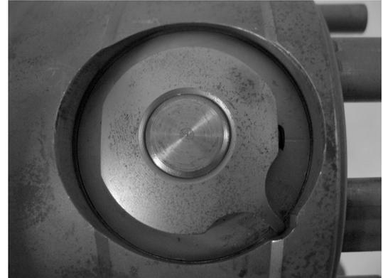
Push the spider gear in until you see the groove where the snap ring will be placed.
