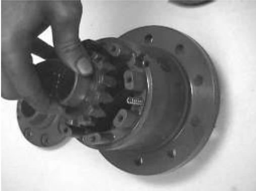
Install locking side gear with gears facing engagement with spider gears
