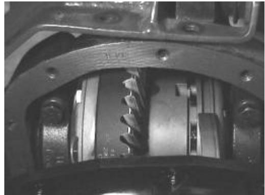
Install cover on to the differential. Make sure the fork slides on the locking ring.
