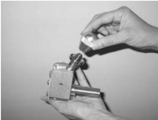
When installing the knob, don't thread all the way down. Make sure that the shifter can shift clear.
