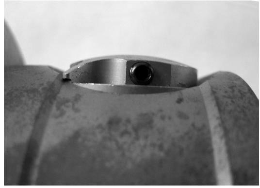
Install the spider gear cap (align the key into the groove in the carrier) – do not push the cap all the way down so that you have room to install the dowel pin.
