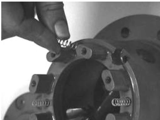
Install the 4 springs in the 4 chamfered holes.
