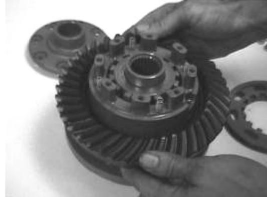
Slide the ring gear around the carrier.
