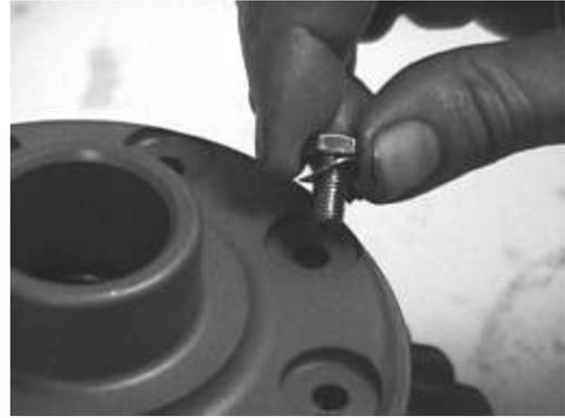
Install the 1/4 bolts and spring washers. Apply high strength loctite to bolts.
