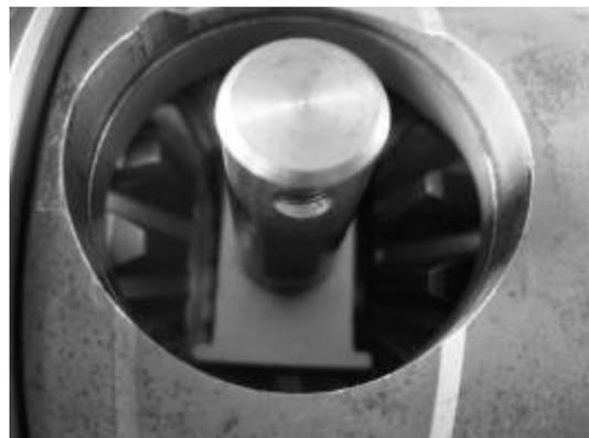
Carefully Install the shaft. The end with the cross hole should be on this end. With the cross hole running north/south and the shaft not be pushed all the way through. Leave some extending out this end to enable you to install the spider gear, cap, dowel pin, and set screw.
