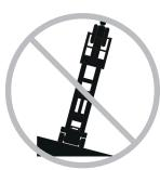
Do not depend on the tilt alarm as a level indicator. The tilt alarm sounds only when the machine is on a slope.
