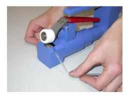
Press the upper handle with strength, while holding the lower handle with the fingers of the same hand.
