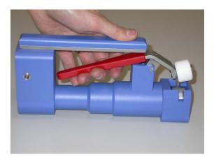
Then press the upper handle as in the photograph. The lower roller (visible only from above) will start turning quickly and with uniform motion.
