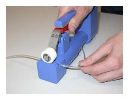
When stripping is finished, release the upper handle.
