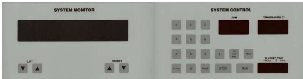
Step 3. Turn on the dissolution apparatus. The red LEDs on the system control panel illuminate. The initial status screen displays for three seconds.
