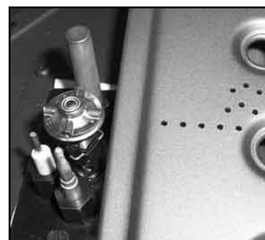
Figure 9. Ignitor assembly beside the burner.
