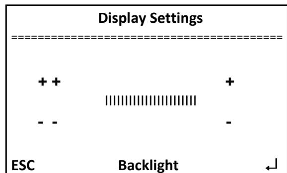
This sub menu allows to set the contrast (Contrast) as well as the reverse light screen (light back). Proceed adjustments with buttons « + », « ++ » and « - » and « - - »
