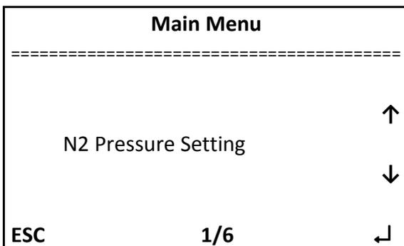
The First menu « N2 pressure setting » (setting of the NITROGEN output pressure) allows as its name indicate to adjust the N2 output pressure.
