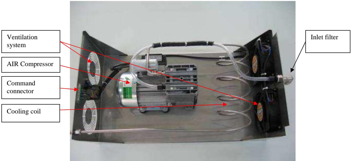
high capacity Air compression module
