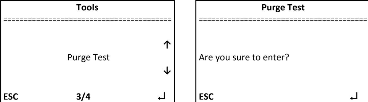
By pressing on key « ↵ » it is possible to enter into the menu and opening or closing the purge.
