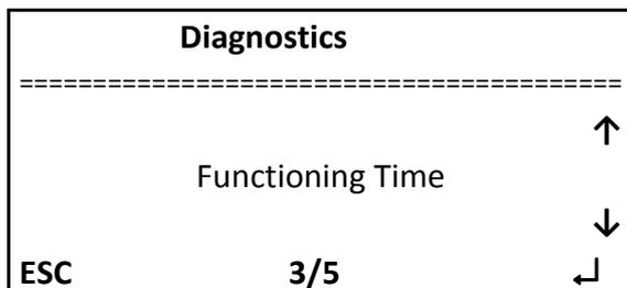
This menu allows **only to observe** the various functioning parameters of the instrument. Moving within the tree is done by using the arrows « ↑ » and « ↓ ». Once the requested setting is found, press on « ↵ » to enter into the sub-menu and « ESC » to come out.
