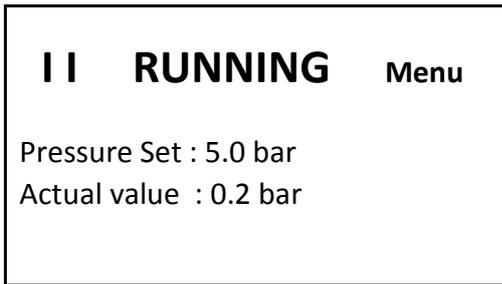
It is possible to check the filling up progression of tank by pressing on MENU then select Diagnostic and Internal Pressure.
