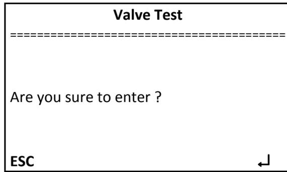
By pressing on « ↵ » It is possible to go into the menu and adjust the setting value
