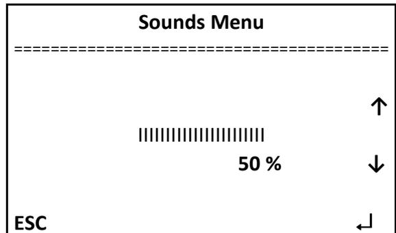
This sub menu lets you adjust the duration of the sound emitted when the screen is touched. A setting to 0 % totally removes the sound.
