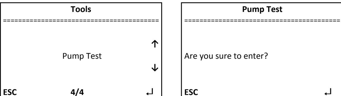
By pressing on key « ↵ » It's possible to enter into the menu and control the start of the compressor as well as checking the Air pressure variation inside the tank.
