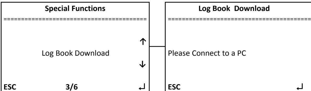
Once the page « log Book Download » is reached, it is necessary to connect the generator to a PC through a USB link. If it's the first time the generator is connected to a PC, he will request to proceed to the set up of the « driver ». It is stored on the CD provided with the instrument in the directory « driver »
