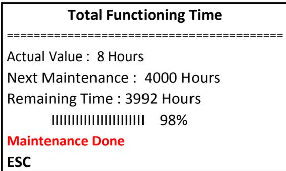
At this time « maintenance done » disappear, the messages « Next maintenance » is incremented by 4000H and the message « Remaining time » is up dated.
