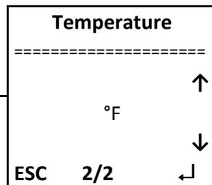
Once in the « UNIT » menu it is possible with the keys « ↑ » and « ↓ » to change the following units : Pressure and Temperature.
