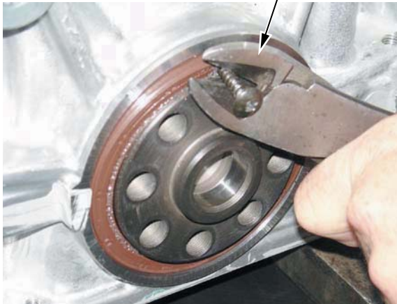
DIAGONAL CUTTERS (Pry out oil seal.)
