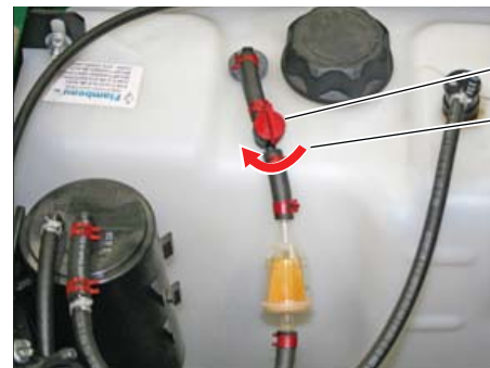
Fuel Shut-off Valve Turn to "OFF" Position
