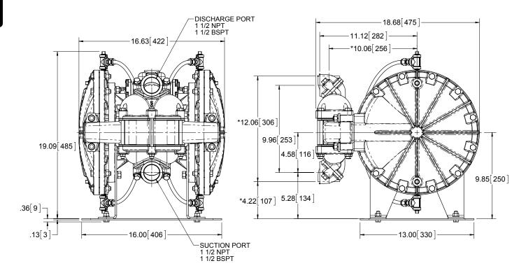
$^{\star}$  INDICATES DIMENSION WITH SUCTION AND DISCHARGE PORTS ROTATED 180  $^{\circ}$  TO A VERTICAL POSITION
