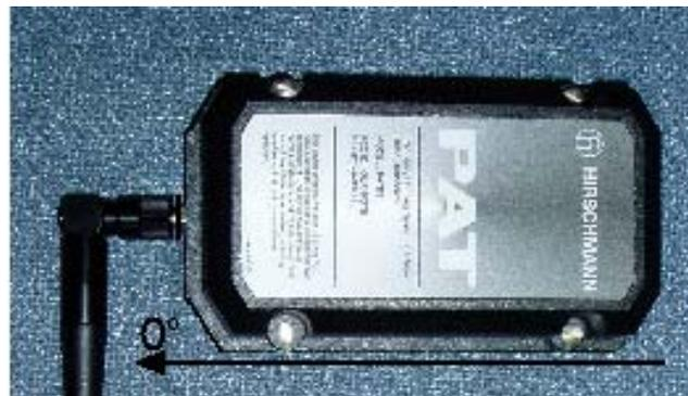
The angle sensor will be mounted on the side of boom so as the boom angle changes, the angle sensor can rotate as shown in the 0° (left) and 90° (above) positions.
