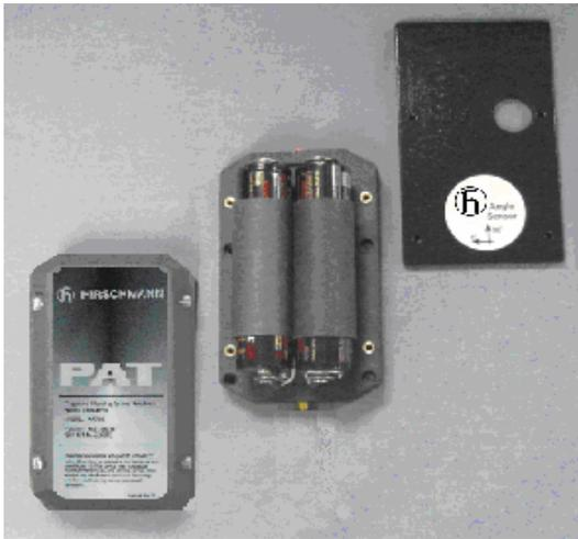
Angle sensor, transmitter, and mounting plate.
