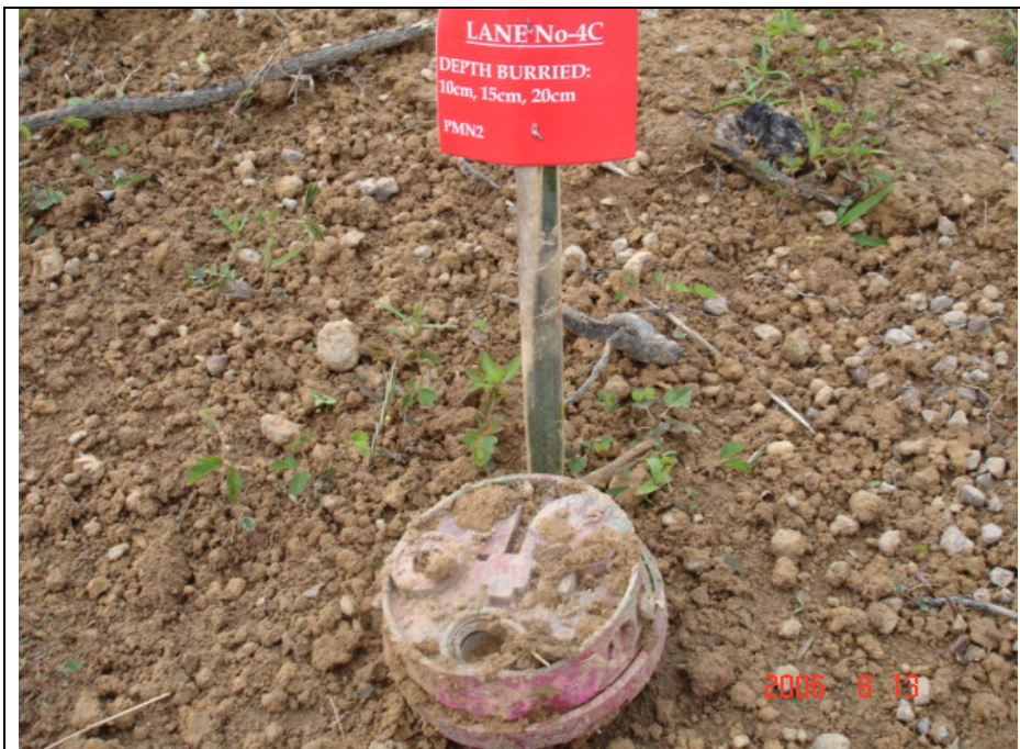
Figure 21: Mine is hit and moved from its original location but still in good condition. This mine is in category three and is subjected for evaluation
