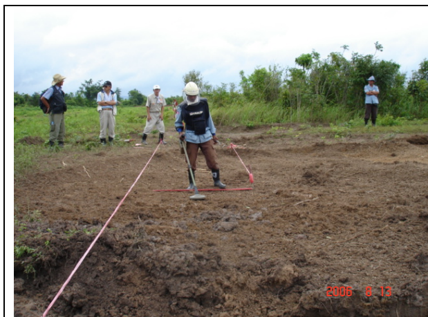
Figure 13: CMAC deminer is using metal detector to re-establish the test lane boundary after the area is cleared by the machine
