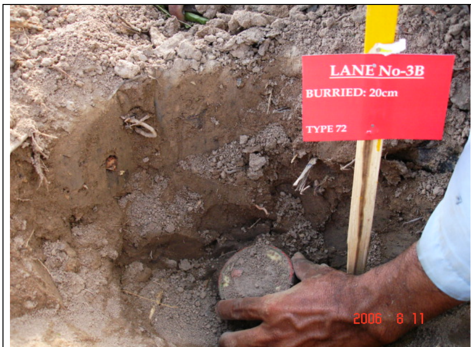
Figure 22: Mine had been hit by the machine but the machine does not have the sufficient digging depth. This mine is subjected for checking
