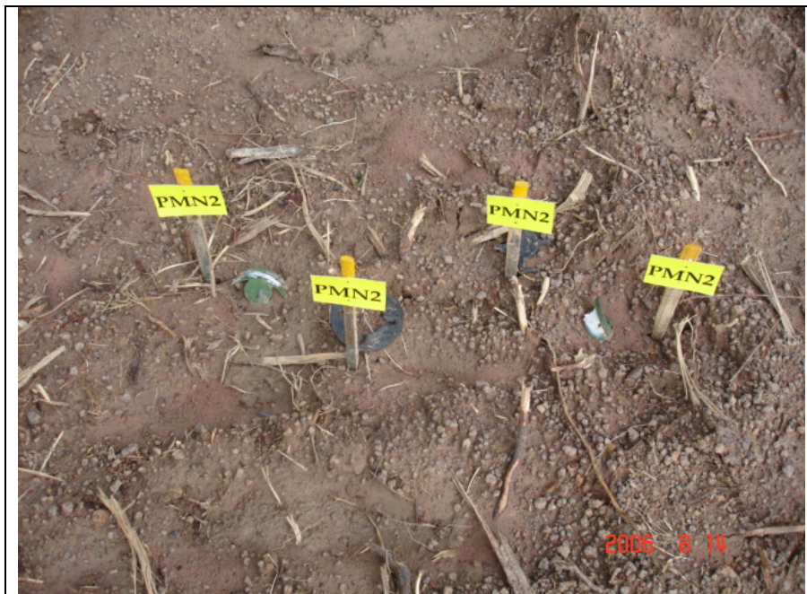
Figure 19: Mine is destroyed by the machine. In this category, mine is classified to be destroyed by the machine.
