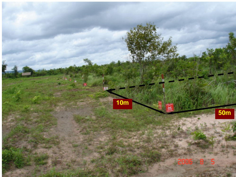
Figure 37: Light Bush test area & test lane arrangement
