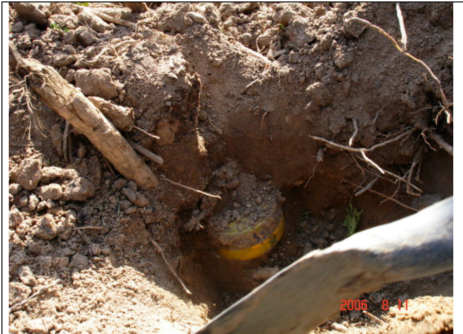
Figure 23: Machine did not touch mine due to insufficient digging depth. Mine still dangerous. Round stick painted in yellow indicate previous mine position.
