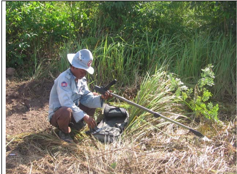
Figure 42: CMAC deminer is setting up metal detector MINELAB F1A4 to be used to remove metallic object from light bush test area.
