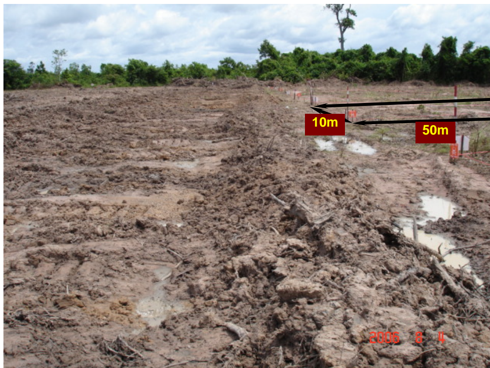
Figure 47: Wet condition test area & test lane arrangement
