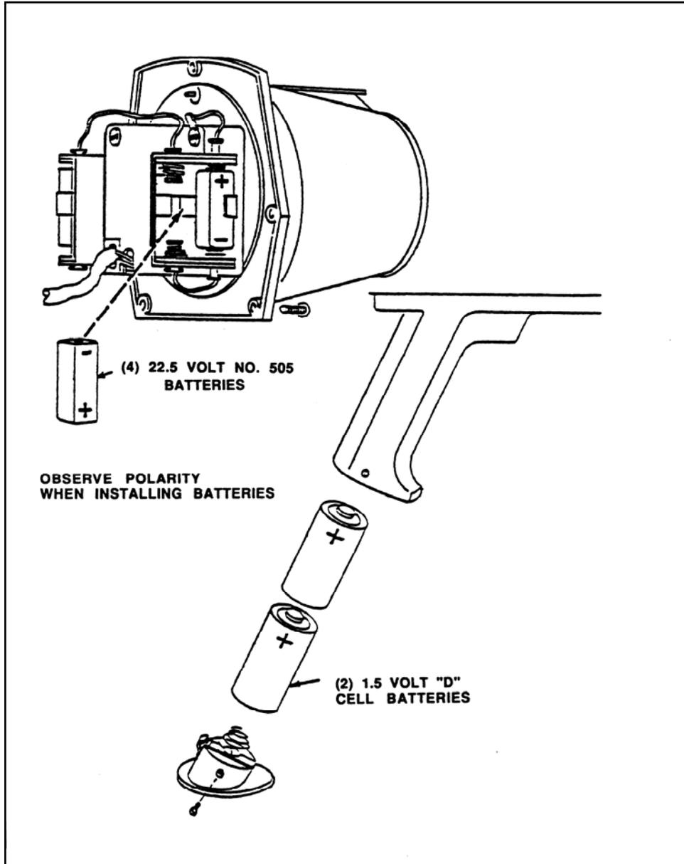
Figure 2-2. Batteries, Cap, and Contact Spring Replacement
