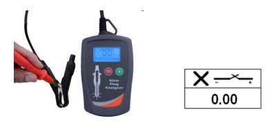
The tester should be checked periodically on its accuracy by shorting the red test probe to the black clamp and the display should show "0.00". In event that it did not, then a zero calibration should be done.
