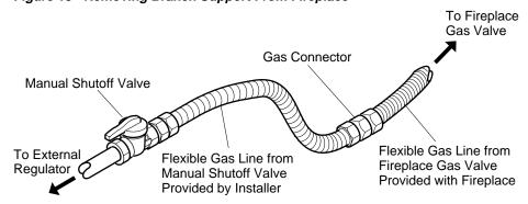
Figure 19 - Attaching Flexible Gas Lines Together
