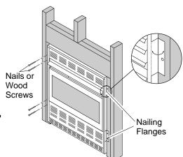
Figure 10 - Attaching Fireplace to Wall Studs
