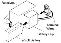
Figure 23 - Attaching Battery to Receiver
