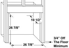
Figure 8 - Rough Opening for Installing in Wall
