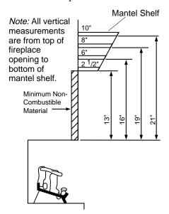
Figure 11 - Minimum Mantel Clearances for Built-In Installation
