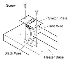
Figure 22 - Switch Plate and Wiring Harness
