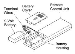
Figure 25 - Installing Battery in Hand-Held Remote Control Unit
