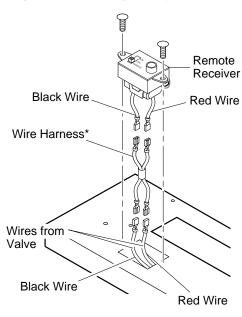
Figure 24 - Installing Remote Receiver
