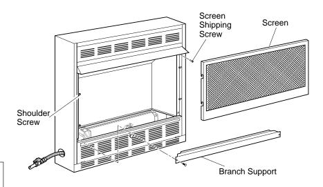
Figure 18 - Removing Branch Support From Fireplace
